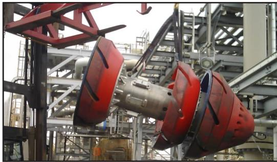
36 IN. MAGNETIC PIG FOR CONDENSATE AND BLACK POWDER REMOVAL.
