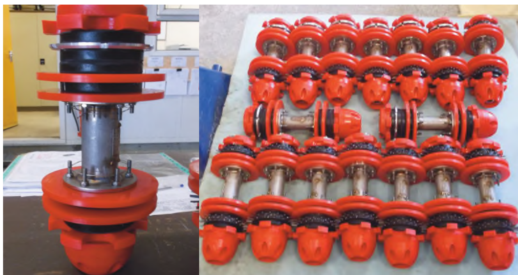
Figure 2. Typical examples of 6 in. cleaning and gauging pigs designed to incorporate four methods of pig tracking/location – neodymium iron boron magnet bracelets, an electromagnetic transmitter, acoustic pinger, radioactive isotope, and smart gauge data logger. The innovative source container is an integral part of the patented wet-buckle insertion tooling design developed for the Ichthys project in Australia.
