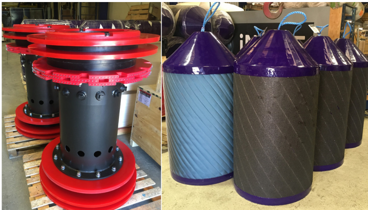
FULL WIRE BRUSH AND CARBIDE FOAM PIGS AND BI-DIRECTIONAL CARBIDE TIPPED STUD PIGS.
